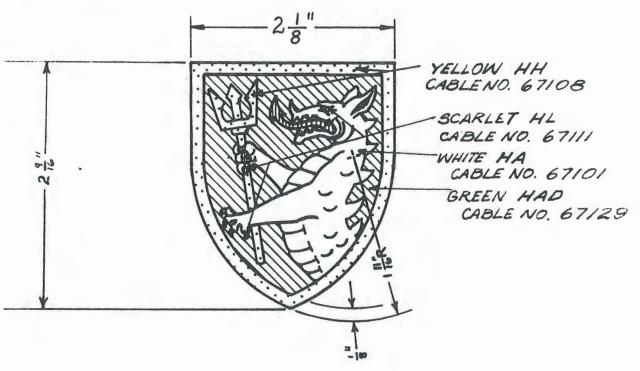
STITCH COUNT 6399 STITCHES (MINIMUM) ALL 100/2 DENIER 12/4 SPAN DESIGNED FOR OVEREDGE STITCHING
